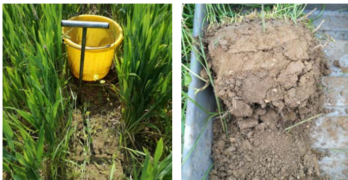
Figure 1: Sampling for lab analyses (left) and structure assessment (right)
