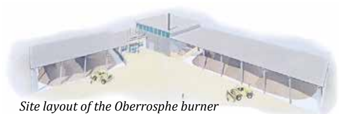
Wood-chip drying undercover before use in the Oberrospe burner to provide heat for 55% of the town's households
