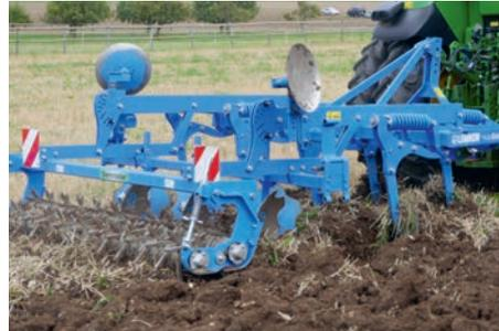
Alternatively to the skim plough a cultivator may be used (picture: a Lemken Terradisc). The duck feet undercut the soil and any docks across the entire working width. The working depth can be adjusted with a support wheel. The cultivator mixes the soil more intensively than the skim plough.
