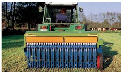
Combined with harrow and roller, slug-pellet spreaders are very well suited for oversowing.
