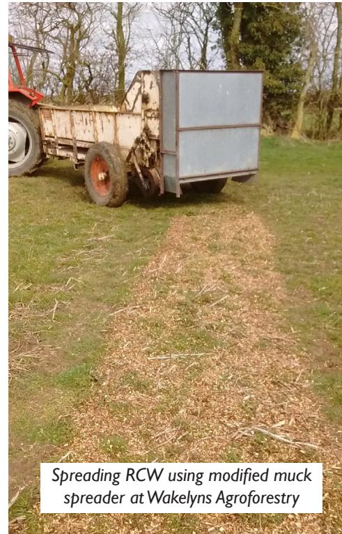
Spreading RCW using modified muck spreader at Wakelyns Agroforestry
