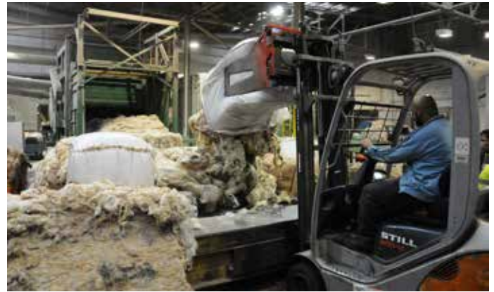
Raw fleece is fed into the scouring unit at Curtis Wool, Bradford
